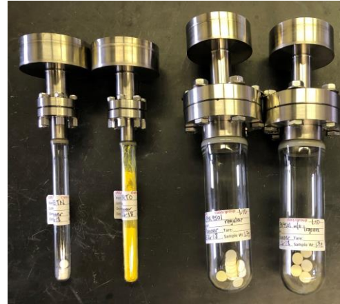
Irradiation vessels containing explosives (inside ammo cans)
