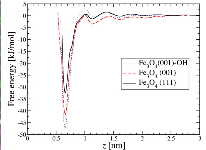
Free-energy profiles as a function of the distance between stearic acid in heptane and the solid Fe<sub>3</sub>O<sub>4</sub> surface calculated using classical MD simulations<sup>2</sup>
