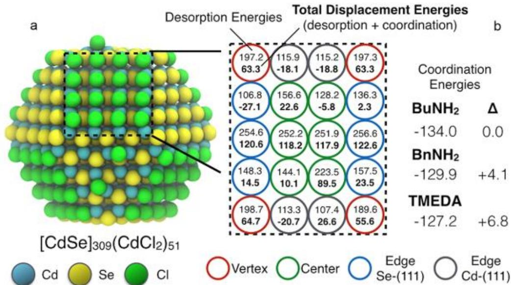
CdCl<sub>2</sub> ligand displacement energies computed at the DFT/PBE level of theory<sup>1</sup>
